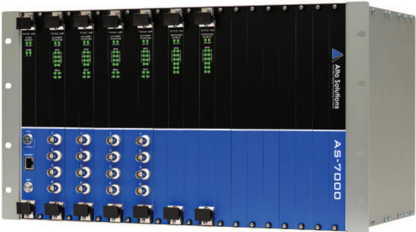
■ The AS-7000 can capture up to 64 dynamic signals using two 24-bit analog-to-digital converters per channel.
